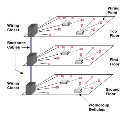
Figure 6: Example of Structured Wiring
