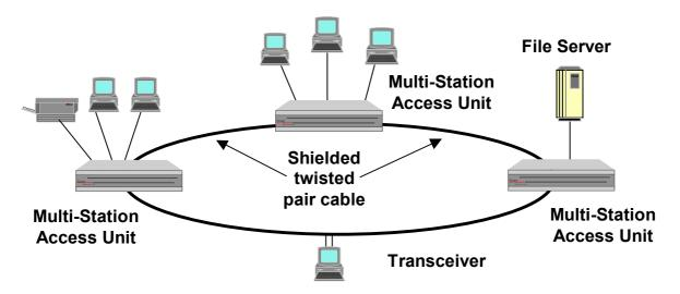
Figure 2: IBM Token Ring Structure
