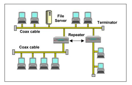
Figure 1: CSMA/CD Tree Structure
