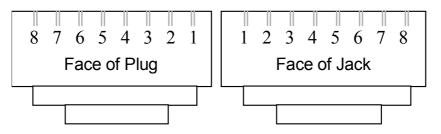
Figure 4: RJ45 Modular Jack Wiring
