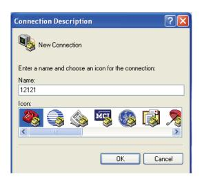
**Step 3** Using Hyper Terminal in Windows for example, as shown to the left. Type in a new name for the connection in the text box "name", then click the "OK" button
