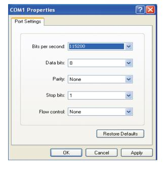
**Step 5** Set the serial port parameters. As shown to the left.
