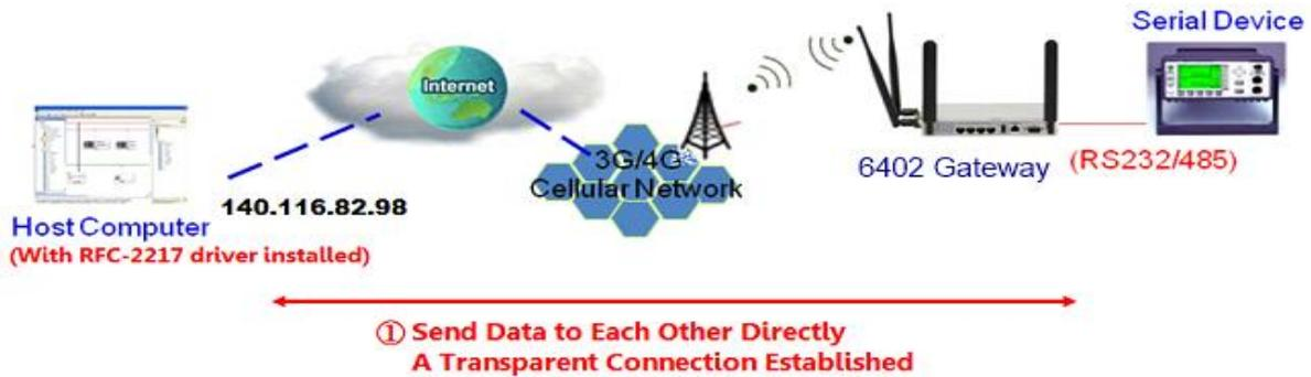
Any 3rd party driver supporting RFC2217 can be installed in the host computer, the driver establishes a transparent connection between host and serial device by mapping the IP:Port of the 6402's serial port to a virtual local COM port on the host computer. The 6402 can support up to 4 remote devices.
